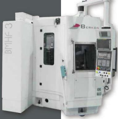
► Special vertical boring machine with two electro-spindles
